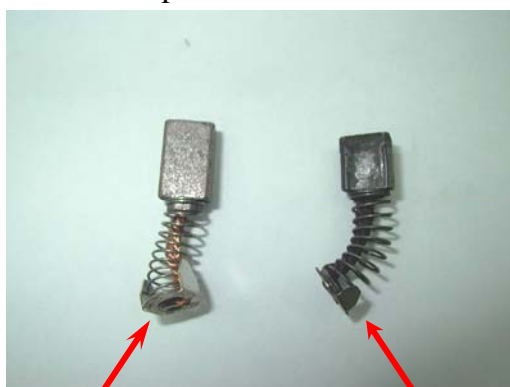
New Motor Brush Worn Motor Brush (Fig 41)
